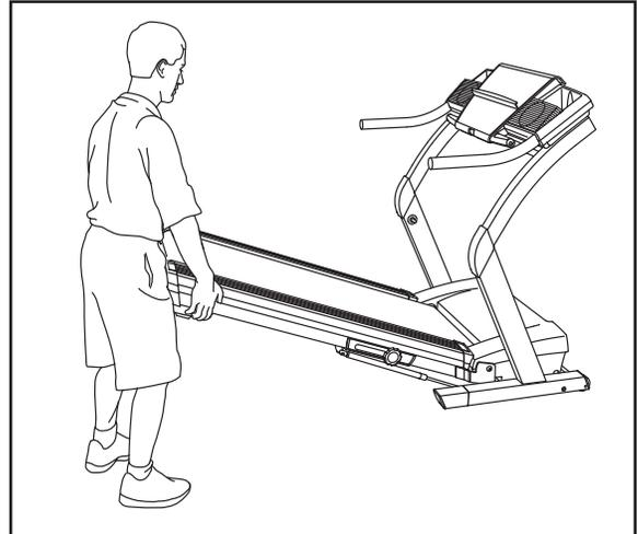
2. Move your right hand to the position shown and hold the treadmill firmly. Using your left hand, pull the lock knob to the left and hold it. Raise the treadmill until the lock pin is aligned with the hole in the housing. Insert the lock pin into the housing. **Make sure that the lock pin is fully inserted into the housing.** Note: If the adjustment knob (not shown) hits the upright, press on the knob.
