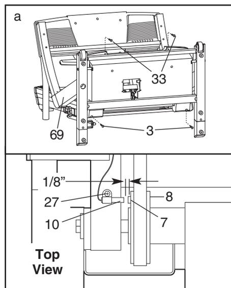
Locate the Reed Switch (10) and the Magnet (7) on the left side of the Pulley (8). Turn the Pulley until the Magnet is aligned with the Reed Switch. **Make sure that the gap between the Magnet and the Reed Switch is about 1/8"**. If necessary, loosen the Screw (27) and move the Reed Switch slightly. Retighten the Screw. Re-attach the hood, making sure the screw are in their same holes. Run the treadmill for a few minutes to check for a correct speed reading.
