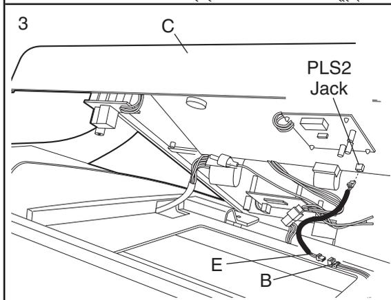
**Make sure that no wires are pinched.** See step 1. Reattach the Console (C) with the screws. **Important: If the screws are not put back into the same holes from which they were removed, the Console will be damaged.**
