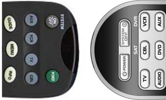
**STEP 2:** On the AVEX R6, press the Component button that you want to program (in this case the button that says TV) and the SELECT [SEL] button at the same time. Hold down both buttons for 2 seconds until the TV Component button light turns on. This signals that you are in programming mode.
