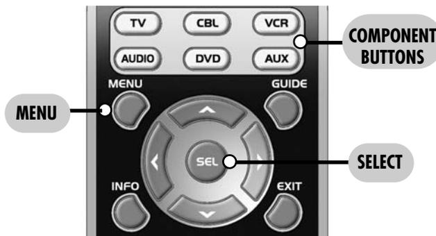
**STEP 3:** Press either the CBL or DVD button that you want to use as the source of OSD Control. The component LED will blink three times to confirm it is saved.
