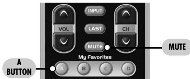
**STEP 3:** Using the Number Pad, punch in the Channel number of the Favorite Channel that you want to store in the Macro button. The Cable component LED light will blink once for each button pressed.
