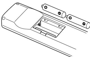
Make sure to match the + and – on the batteries to the marks inside the battery compartment.
