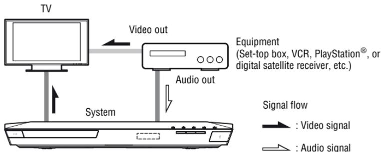
Select one of the following connection methods according to the jack type of the equipment.
