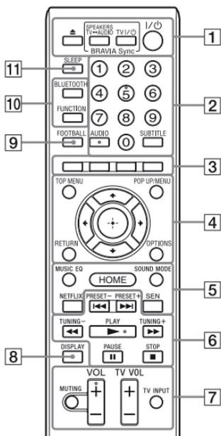
Number 5, AUDIO, VOL +, and ► buttons have a tactile dot. Use the tactile dot as a reference when operating the remote control.
