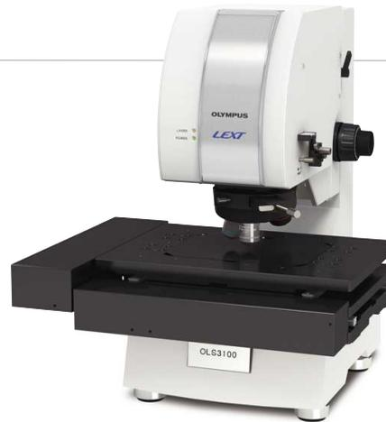
Configuration with a motorized stage
