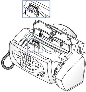
**Insert the Cartridge in the Carrier**, then push it firmly until it clicks into place. If the Cartridge moves loosely in the Carrier, it has not clicked into place. Repeat this step.
