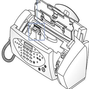
**Re-install the Cartridge** and close the Cover and Panel.
