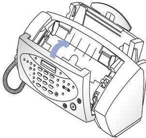
**Replace the Cartridge Compartment Cover and Control Panel.**
