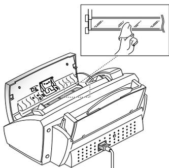
**Carefully wipe the Scanning Glass** with a soft, dry cloth. If the glass is very dirty, first wipe it with a slightly dampened cloth, then with a dry one. Be careful not to scratch the glass surface.
