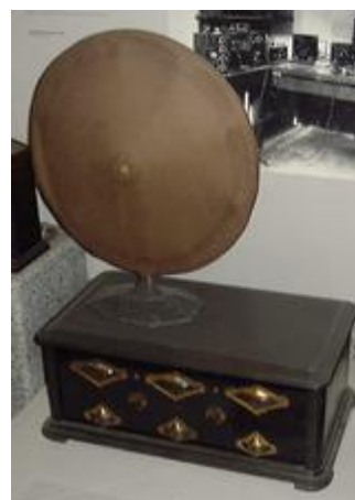
1925 Grebe radio receiver and 1924 Western Electric 540 speaker (NMAH)
