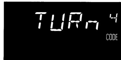
**Step 6:** When 1/2 the defrosting time is completed, the oven signals and "TURN" flashes on display instead of time counting down. Open door and turn package over.
