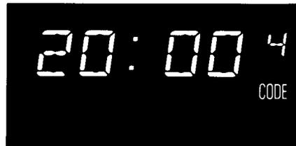
**Step 8:** When defrosting time is completed, oven automatically switches to a Hold period of 20 minutes for code 4. Hold time counting down shows on display. When holding time is finished oven signals, "End" flashes, and oven turns off.
