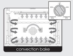
more juices and natural flavor on the inside with less shrinkage. This even circulation of air equalizes the temperature throughout the oven cavity and eliminates the hot and cold spots found in conventional ovens.
