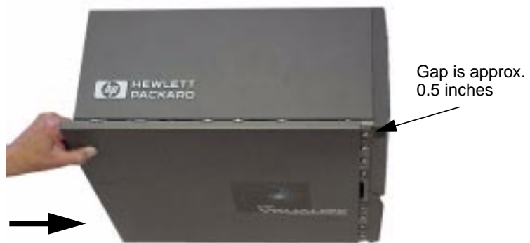
Figure 2-19 Sliding the Left-Side Panel into Place
