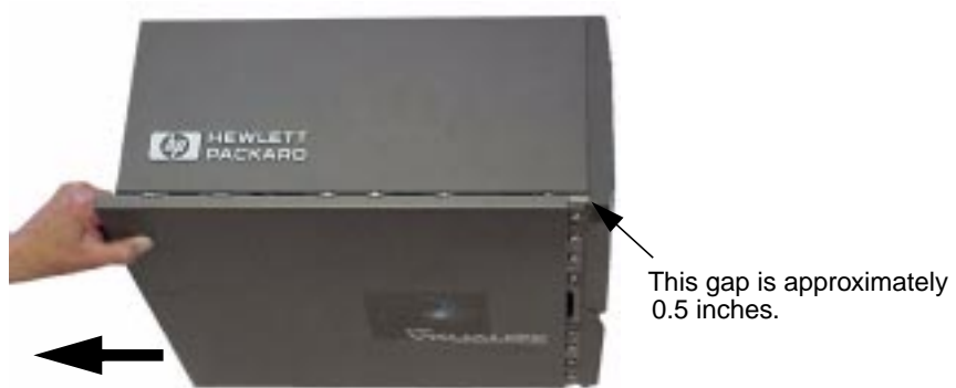
Figure 2-2 Sliding the Left-Side Panel to the Rear of the Personal Workstation
