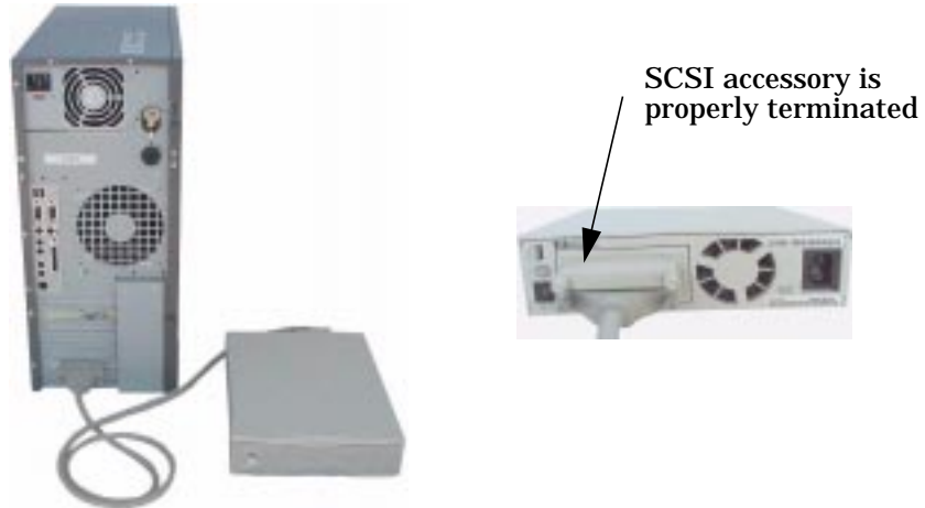
Figure 1-9 Terminating the SCSI Accessory
