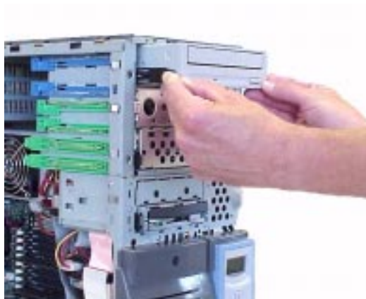
Figure 2-41 Remove the CD Drive into the Top Shelf
