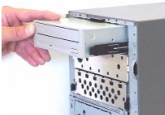
Figure 2-34 Install the CD Drive into the Top Shelf
