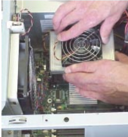
Figure 2-87 Installing the Processor Fan Mount
