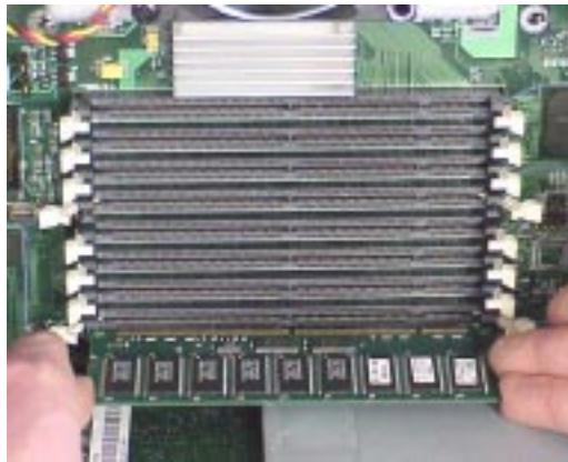
Figure 2-26 Lifting the DIMM Card Out of the Personal Workstation
