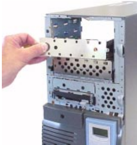
Figure 2-31 Removing the Metal Blank from the Accessory Chassis
