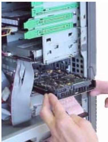
Figure 2-64 Remove the Hard Disk Drive from Its Shelf
