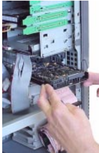
Figure 2-54 Install the Hard Disk Drive into Its Shelf
