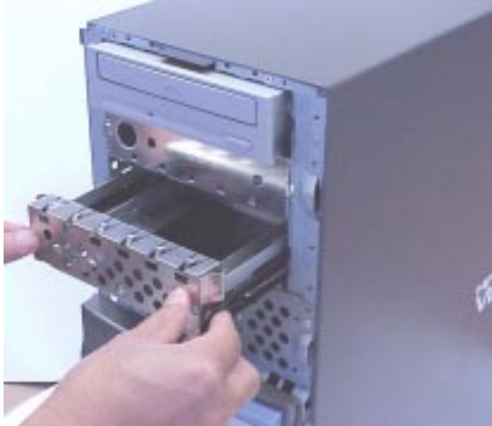
Figure 2-71 Install the Hard Disk Drive Mounting Bracket
