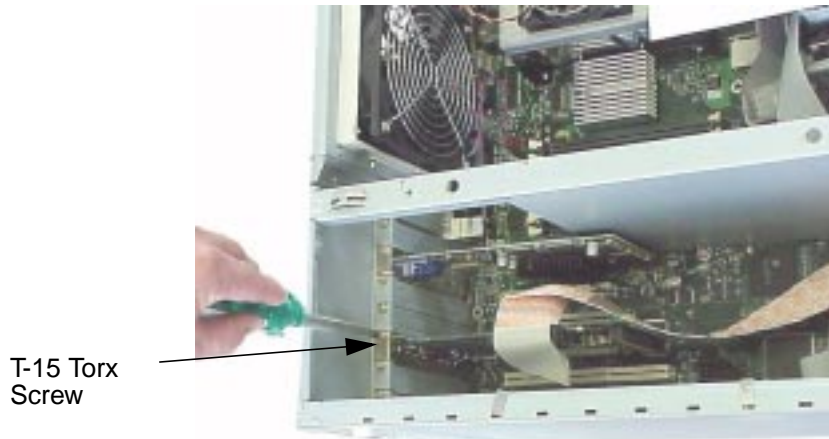
Figure 2-77 Completing the I/O Card Installation
