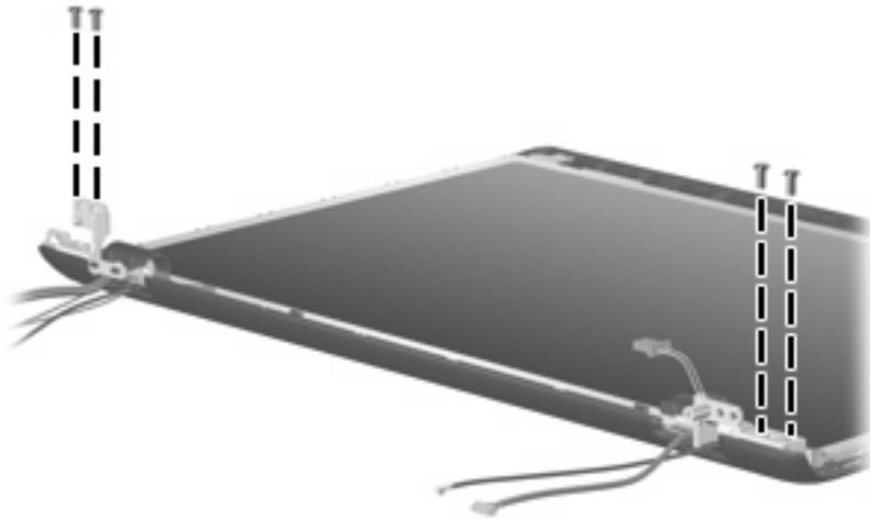
**Where used:** 4 screws that secure the display hinges to the display enclosure
