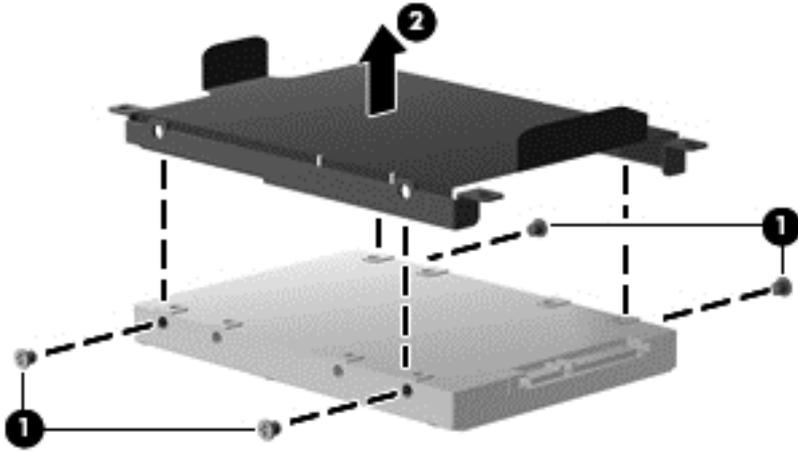
Reverse this procedure to install the hard drive.
