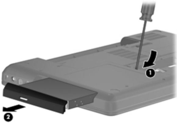
4. To replace the optical drive bracket, position the optical drive with the optical drive bracket toward you.
