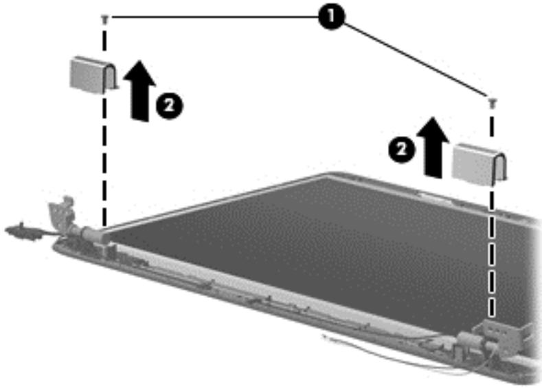
5. Remove all screws (1) that secure the display panel assembly to the display enclosure.
