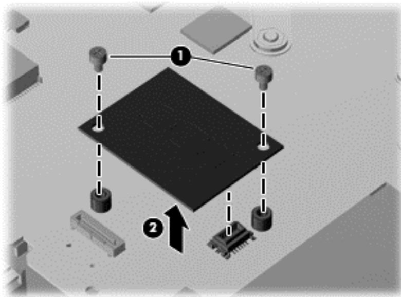
Reverse the above procedure to install the modem module, and be sure that the connector on the bottom of the modem module connects firmly into the system board.
