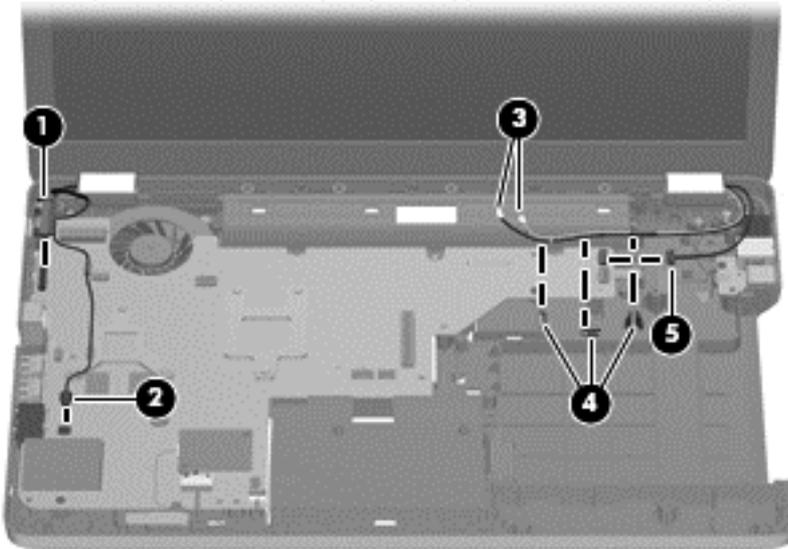
6. Remove the six black Phillips PM2.5×7.0 screws (1) that secure the display assembly to the computer.
