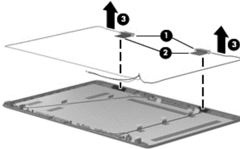
Reverse this procedure to install the display wireless antenna transceivers.
