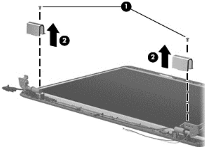
Reverse this procedure to install the display hinge covers.
