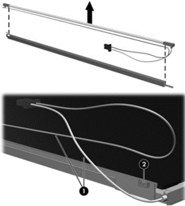
18. Disconnect the display cable (1) from the LCD panel.
