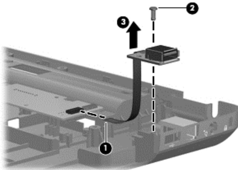
Reverse this procedure to install the USB board.
