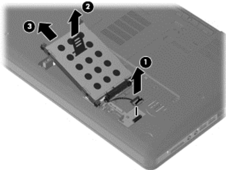
6. To replace the hard drive bracket, remove the four Phillips PM3.0x4.0 screws (1) that secure the hard drive bracket to the hard drive
