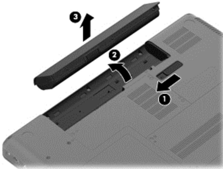
To insert the battery, insert the rear edge of the battery into the battery bay and pivot the front edge downward until the battery is seated. The battery release latch automatically locks the battery into place.
