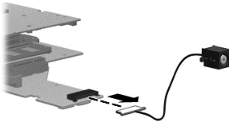
Reverse this procedure to install the power connector.
