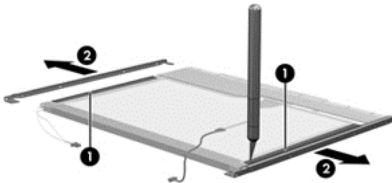
10. Remove the screws (1) that secure the backlight cover to the display panel.
