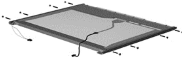
8. Use a sharp-edged tool to cut the tape (1) that secures the sides of the display panel to the display panel frame.
