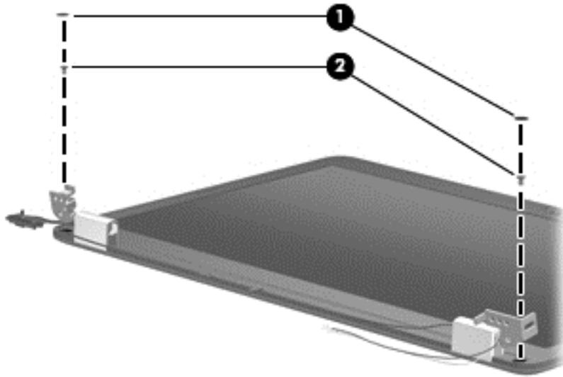
2. Lift up and out on the left and right inside edges (1) and the top and bottom inside edges (2) of the display bezel until the bezel disengages from the display assembly.
