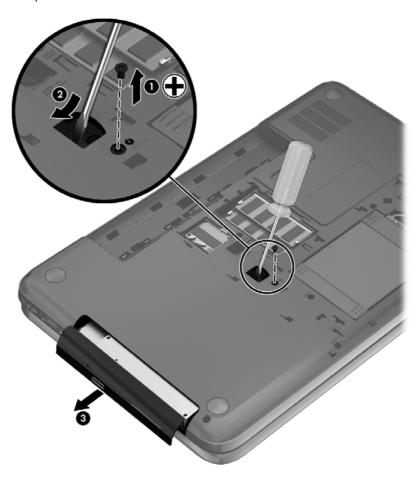
4. Remove the 2 PM 2.0 x 3.0 screws (1) that secure the optical drive bracket to the optical drive and then remove the bracket (2) from the optical drive.
