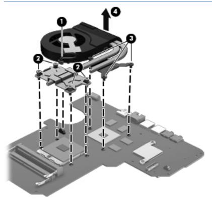
NOTE: The thermal material must be thoroughly cleaned from the surfaces of the heat sink and the system board components each time the heat sink is removed. Replacement thermal material is included with the base enclosure, heat sink, processor, and system board spare part kits.
