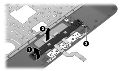
Reverse this procedure to install the TouchPad button board and cable.
