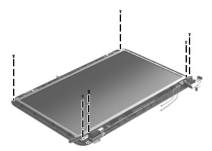
**b.** The hinge covers are held in place by two of the same screws as the display hinges. Using a small tool to pry, remove the hinge covers.
