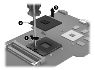
Reverse this procedure to install the processor.
