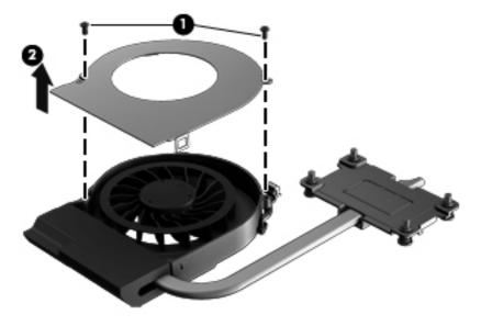
Reverse this procedure to reassemble and install the fan and heat sink.
