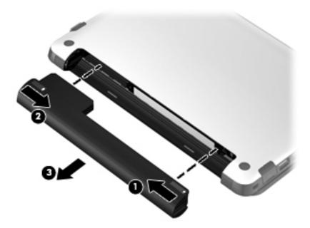
Reverse this procedure to install a battery.
