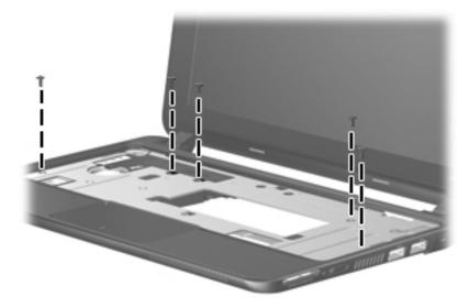
8. Release the top cover (1) by lifting the rear edge until it disengages from the base enclosure.
