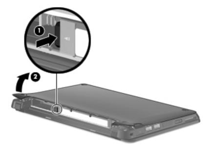
5. Continue lifting the rear edge of the service cover (1) up and forward until it rests at an angle, and then remove the service cover (2).
