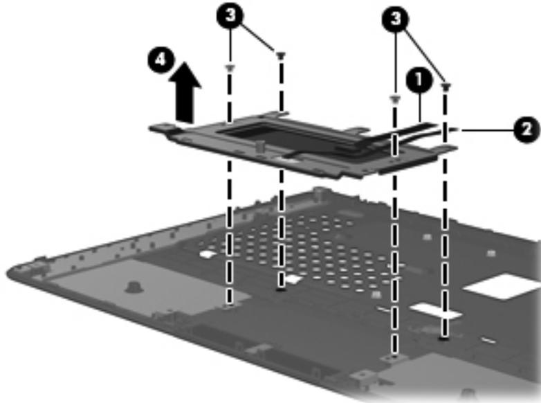
Reverse this procedure to install the TouchPad button board and cable.
