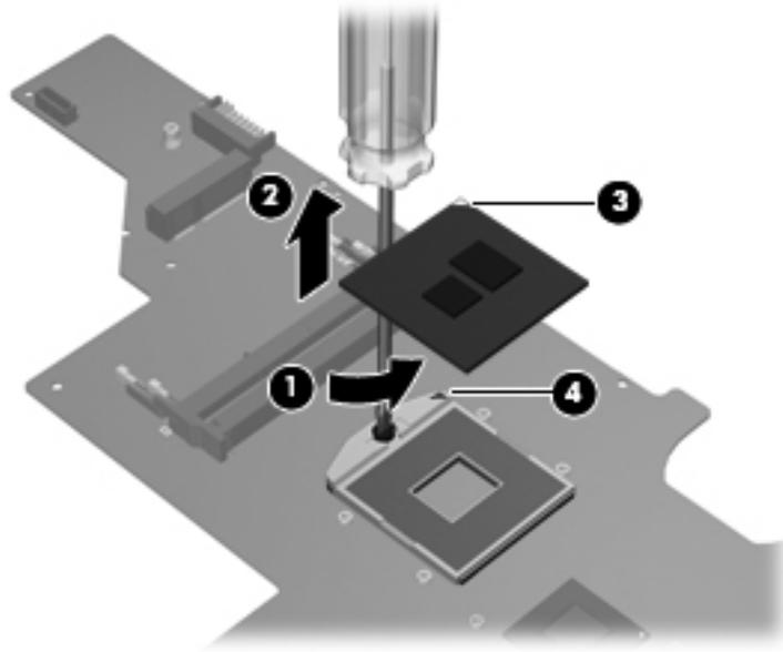
Reverse this procedure to install the processor.
