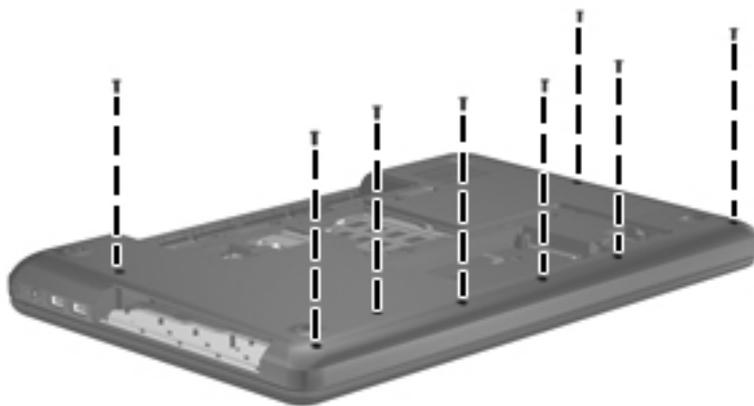
4. Remove the seven Phillips PM2.5×6.0 screws in the battery bay and the hard drive bay that secure the top cover to the computer.
