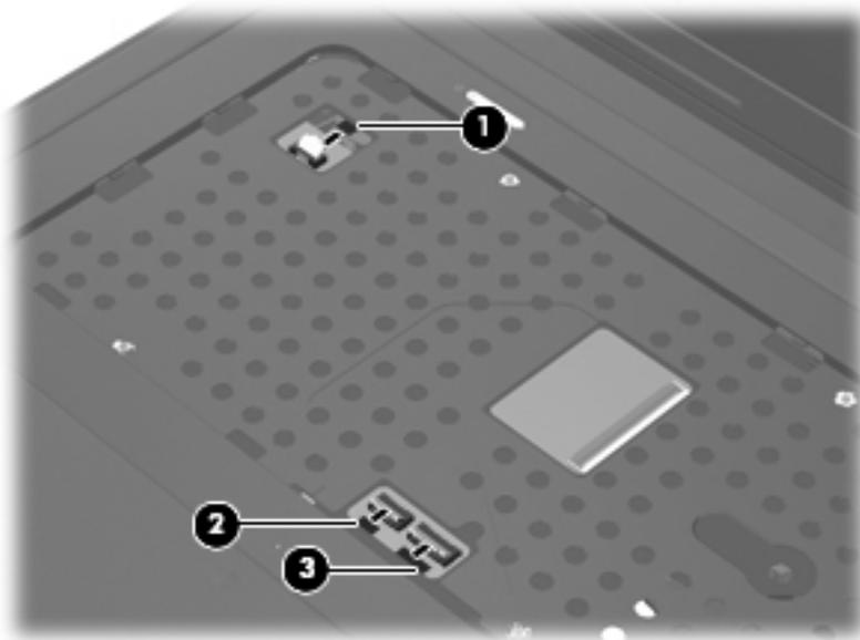
9. Remove the Phillips PM2.5×6.0 screw that secures the top cover to the computer.
