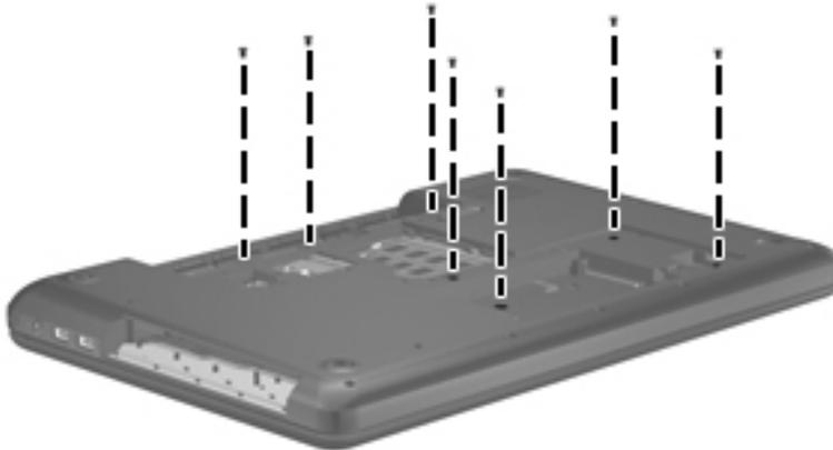
5. Remove the two Phillips PM2.5×9.0 screws **(1)** and the three Phillips PM2.0×3.0 screws **(2)** in the battery bay that secure the top cover to the computer.
