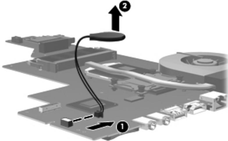
4. Remove the RTC battery.
