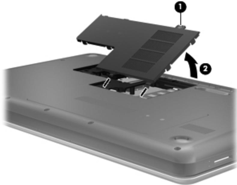
3. Remove the memory module/wireless module compartment cover. The memory module/wireless module compartment cover is available in the Plastics Kit, spare part number 646131-001.
