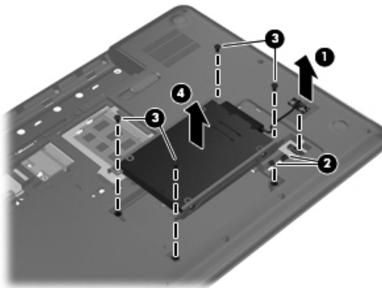
8. If it is necessary to replace the hard drive connector cable **(1)**, the hard drive screws **(2)**, or the hard drive bracket **(3)**, remove and replace the components.
