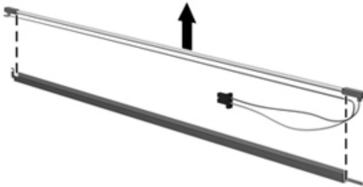
**19.** Disconnect the display cable **(1)** from the LCD panel.
