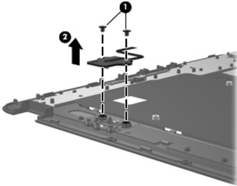
Reverse this procedure to install the power button board and cable.
