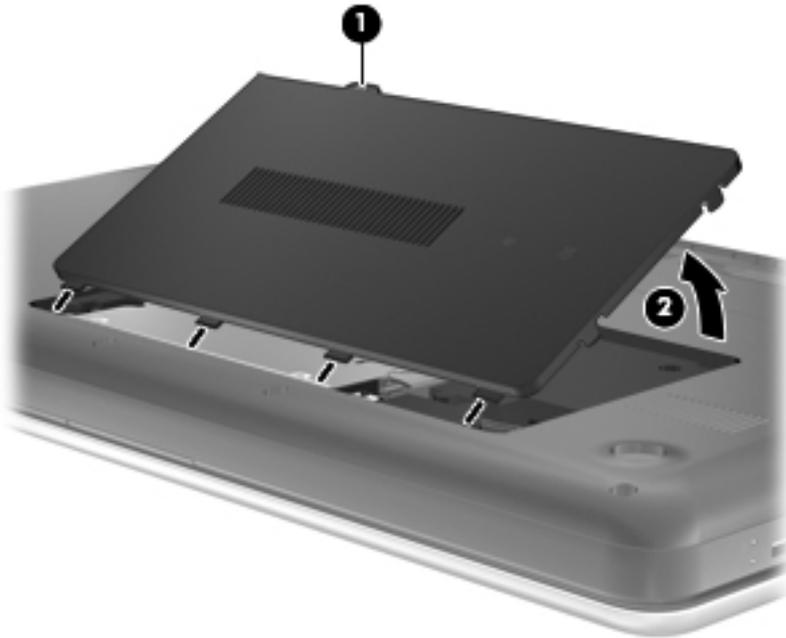
3. Remove the hard drive compartment cover. The hard drive compartment cover is available in the Plastics Kit, spare part number 646131-001.
