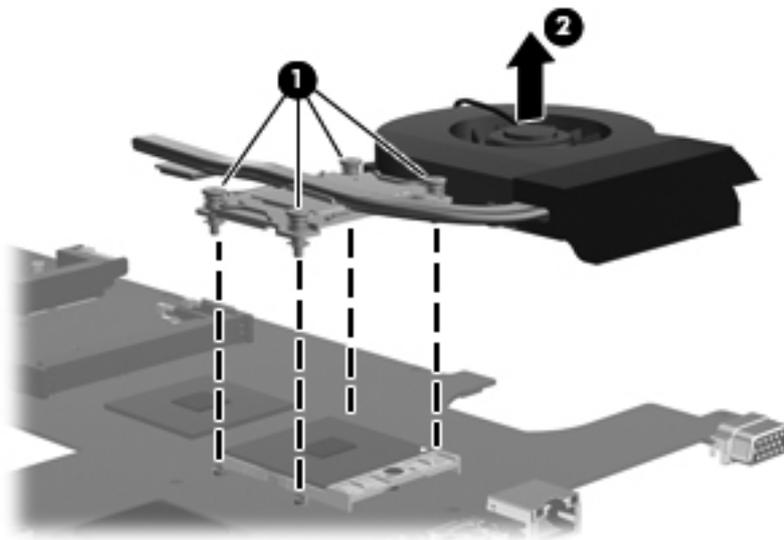
The thermal material must be thoroughly cleaned from the surfaces of the heat sink and the system board components each time the heat sink is removed. Replacement thermal material is included with the base enclosure, fan/heat sink assembly, processor, and system board spare part kits.
