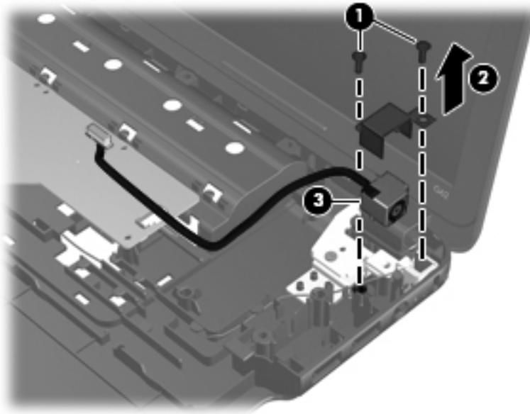
Reverse this procedure to install the power connector cable.
