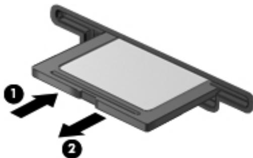
**NOTE:** If the card is not ejected, pull the card out of the slot.
