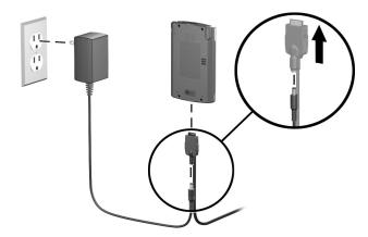
4. When instructed by **Setup Wizard**, connect the HP iPAQ to the computer by inserting the USB plug on the sync cable into a USB port on your computer.
