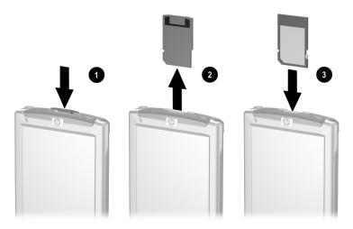
3. When the protective card disengages and pops up **2**, remove it from the expansion slot.
