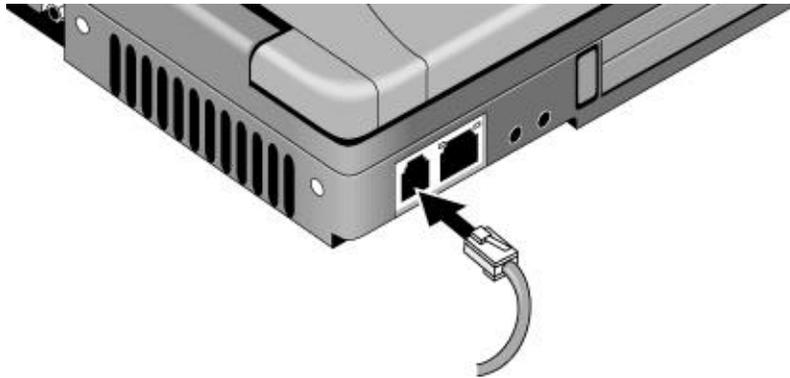
3. Plug the other end of the cord into a telephone jack. If the plug on the phone cord doesn't fit your telephone jack, you may need to use an adapter.
