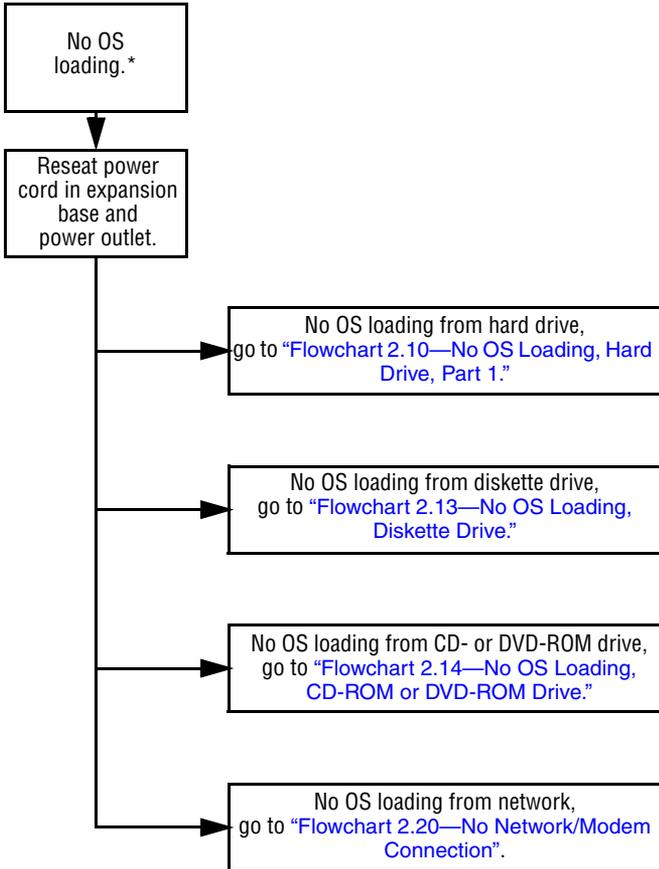
\*NOTE: Before beginning troubleshooting, always check cable connections, cable ends, and drives for bent or damaged pins.
