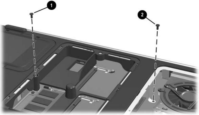
*Removing the Keyboard Screws*
