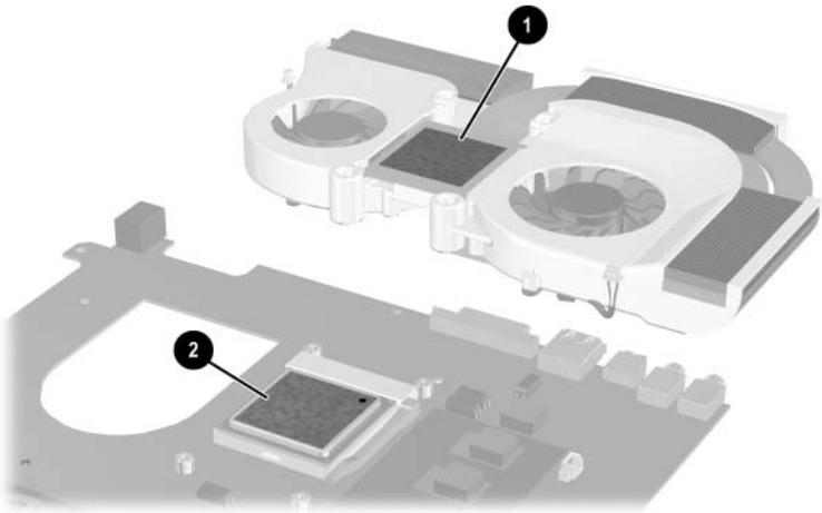
*Removing the Thermal Paste from the Heat Sink and Processor*
