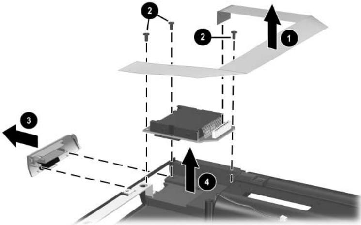
*Removing the SD Card Slot/Infrared Module*
