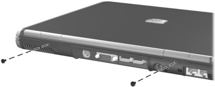
*Removing the Display Assembly Screws*
