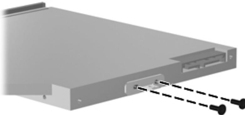
**Where used:** 2 screws that secure the optical drive bracket to the optical drive
