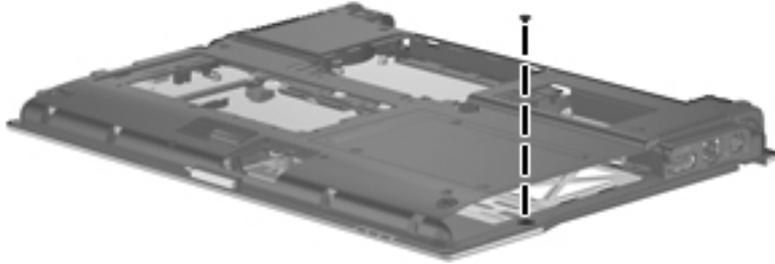
**Where used:** One screw that secures the top cover to the base enclosure
