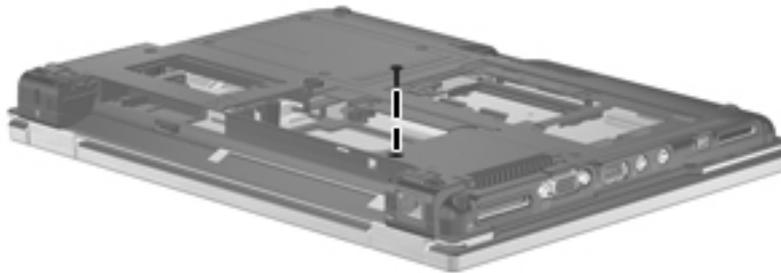
**Where used:** One screw that secures the switch cover to the base enclosure
