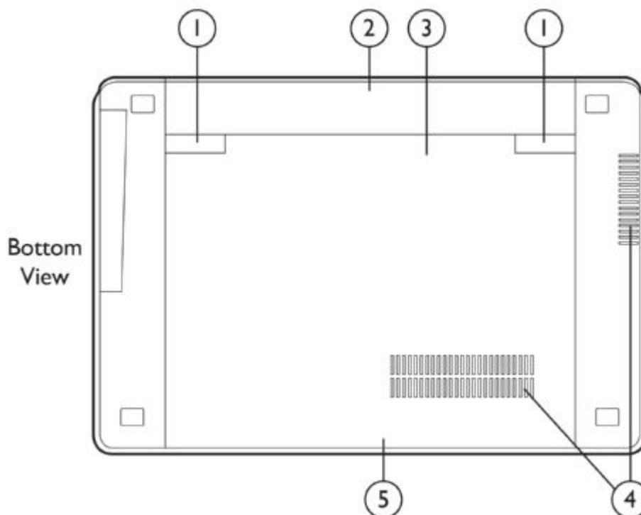
1. Battery and access cover release latches
