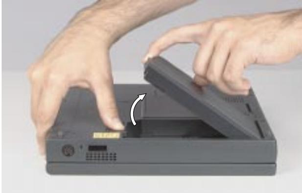
6. Place the fresh battery pack into the battery bay, pushing downward until it snaps into place.
