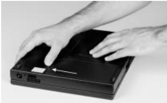
5. Hold the latch back and lift the battery up out of the battery opening.
