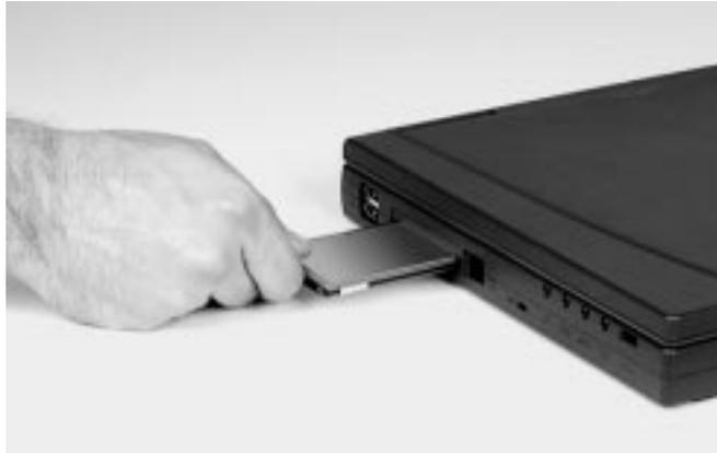
When a card is installed, the eject button can be folded into the system to prevent breakage.
