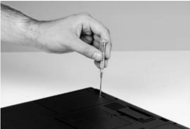
8. Gently pry the hard disk drive latch up and out of the seated position. Slide the hard disk drive forward and lift it out of the hard disk drive tray.
