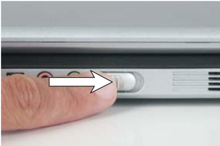
The power switch is preset to On/Off mode. However, you can also set it to function in Standby/Resume mode. For instructions on changing the power switch mode, see [“Changing power settings” on page 165](#).
