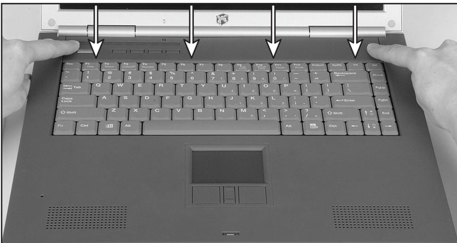
The bezel is correctly mounted when you can run your finger along the bezel and find no loose spots. The bezel should be flat all the way across. If the bezel is mounted incorrectly, complete the instructions under “Replacing the bezel” on page 9.
