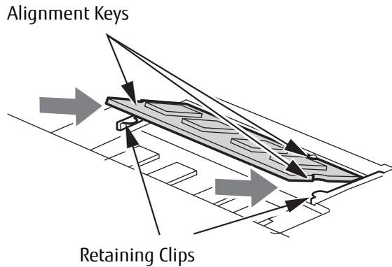
**Figure 29. Installing memory module**
