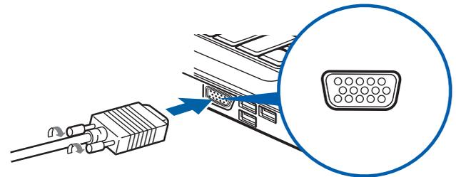
Figure 33. Connecting an External Video Device
