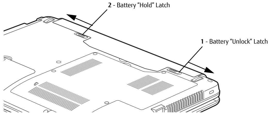
**Figure 21. Battery latches**
