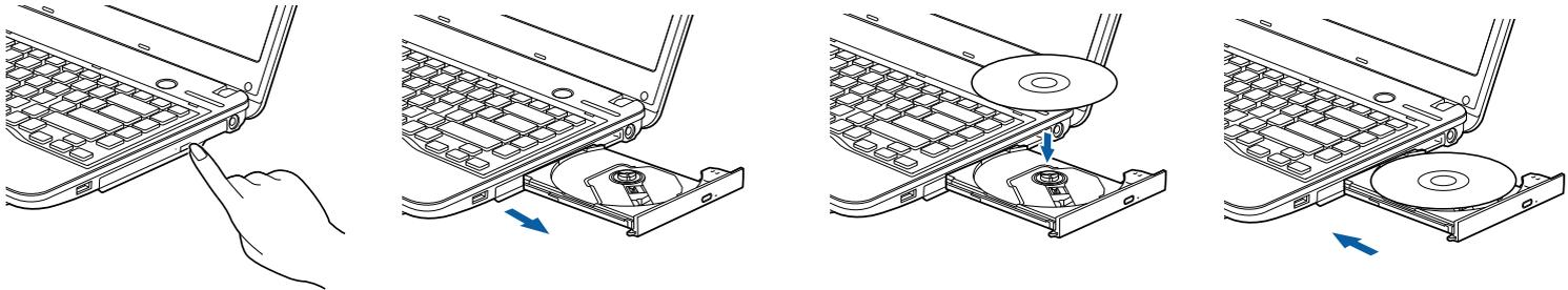
**Figure 24. Loading/Ejecting Media**
