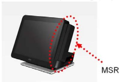
2. Move the magnetic stripe card in the direction of the arrow. Move the magnetic card from the far end of the slot to the front.
