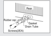
**Installation of the Drain Tube** Fix the drain tube as shown in the figure.
