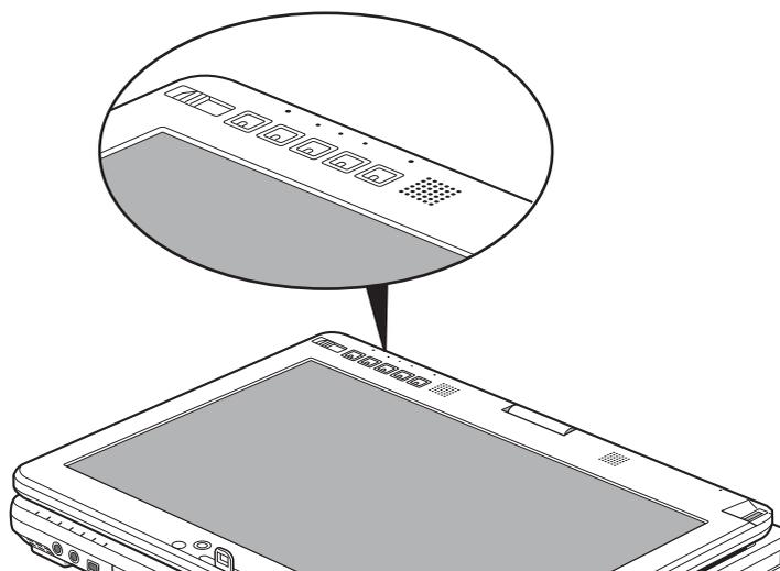
**Figure 33. LifeBook T730 Tablet PC Security/Tablet PC Buttons**
