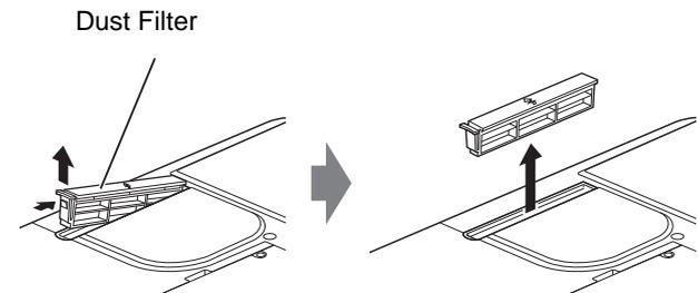
Figure 49. Removing the dust filter
