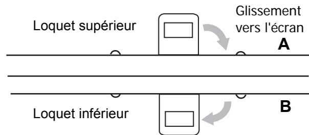
**Figure 9. Verrouillage/Déverrouillage**
