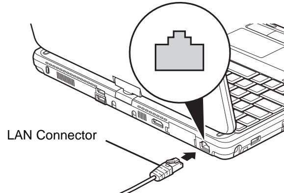
**Figure 44. Connecting the LAN**
