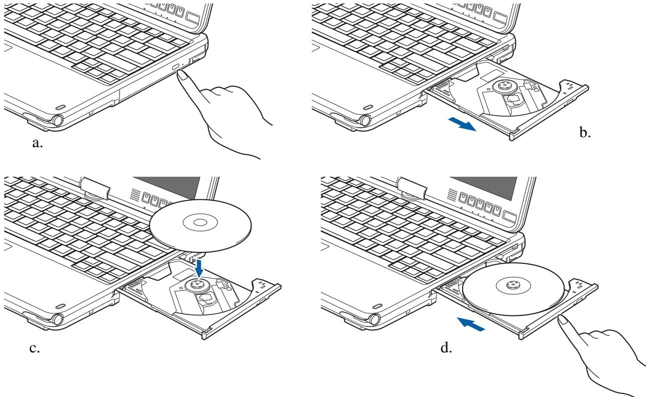
**Figure 42. Loading/Ejecting Media**
