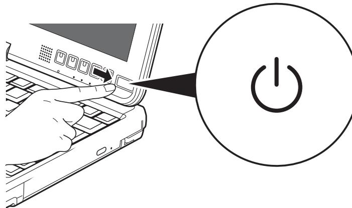
**Figure 35. Power/Suspend/Resume Switch**
