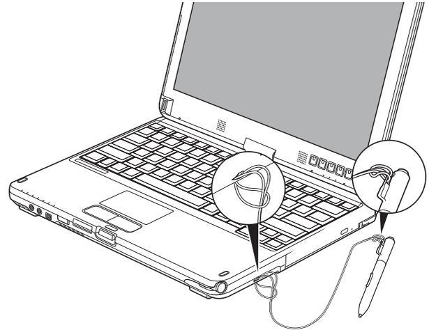
**Figure 30. Installing a Pen Tether**
