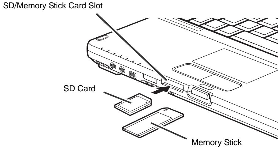
**Figure 37. Installing a Memory Stick or SD Card**
