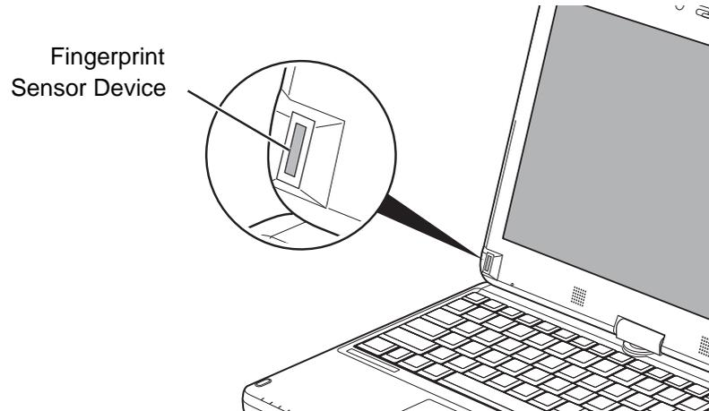
**Figure 53. Fingerprint sensor**
