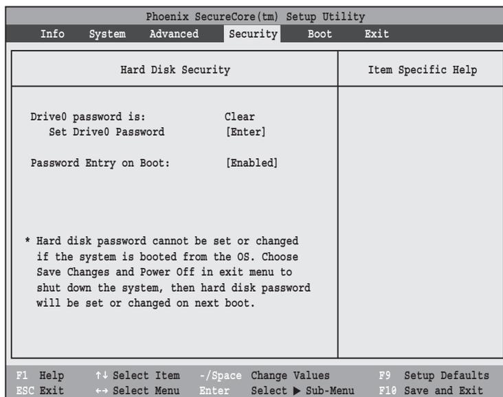
Figure 14. Hard Disk Security Submenu
