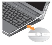
To eject a disc from the drive, gently touch the eject control . The control will flash to confirm for a few seconds before ejecting the disc.
