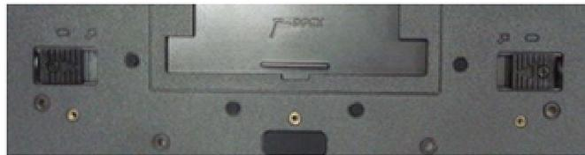
Battery release latches in locked position
