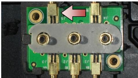
3. Connect the antenna connections to the RF Passthru board.
