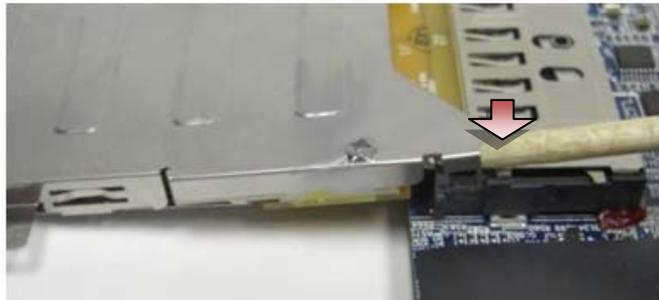
**🔩 NOTE:** Do NOT remove the two screws on the upper back corners of the card cage. They are used for retaining the card cage to the card extender board.
