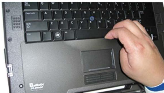
3. After the middle is separated from the palm rest, peel the overlay from middle to left.
