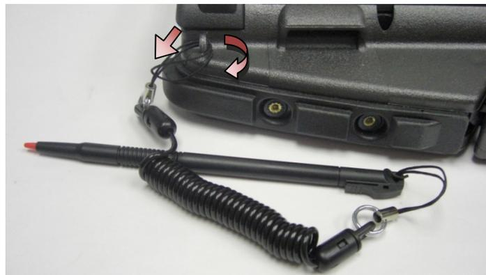
4. Once the stylus and tether are completely through the tether loop, pull the stylus to secure the tether loop onto the tether anchor.
