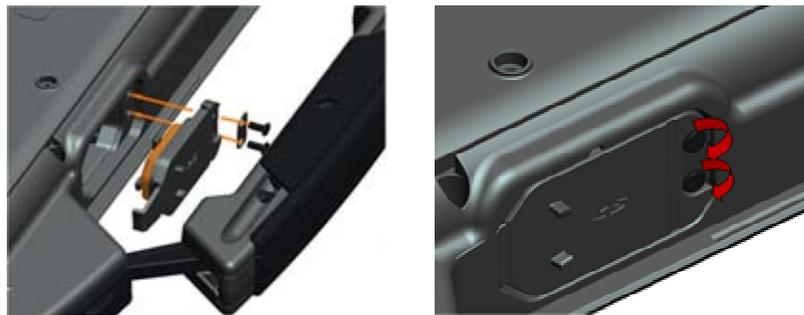
3. Replace the handle (see [Replacing the Handle](#))
