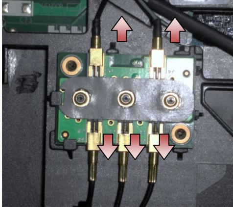
4. Gently lift the lower-right corner of the RF Passthru board, and remove the RF Passthru board by sliding it out of the chassis socket.
