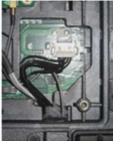
11. Connect the display cable to the display cable connector on the system board.
