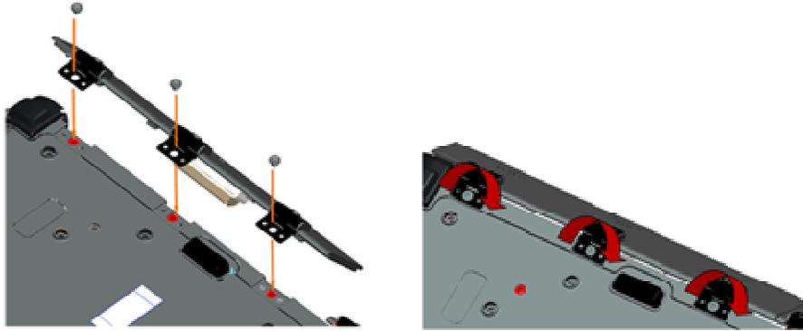
2. Insert the three M3 x 3-mm screws and fit securely.
