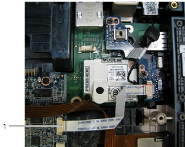
1 Wi-Fi Sniffer cable connection to motherboard
