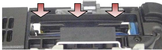
5. Remove the smartcard connector from the system board.
