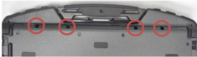
4. Place a scribe against the handle socket on the side, press in 1 inch and rotate to the front to lift the palm rest area slightly.
