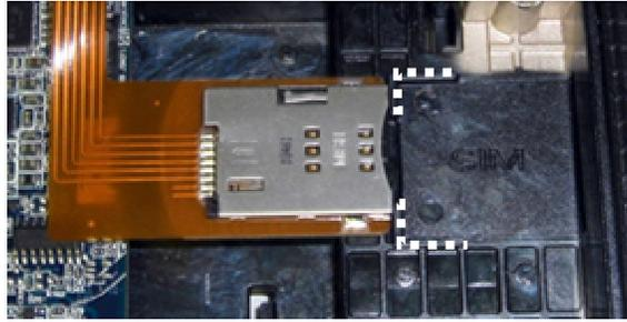
3. Route the SIM extension cable and reconnect the SIM extension board into the original SIM slot located in the battery bay.
