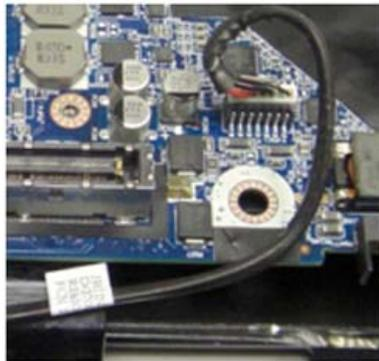
19. Lift the system board out of the base assembly.
