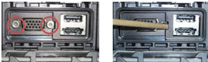
3. Remove the two VGA Connector socket screws.
