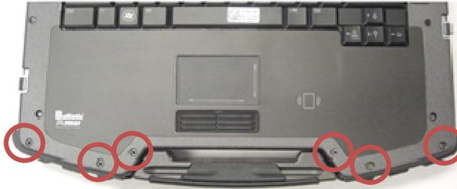
3. Turn the system over and remove the four M2.5 x 8-mm palm rest retainer screws.
