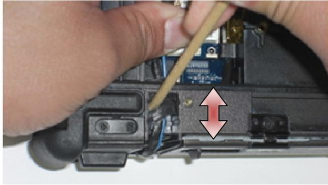
On the LVDS connector, rotate the blue pull-tab used to disconnect the cable from the system board to wrap the cable-side of the connector when routing through the chassis bridge.
