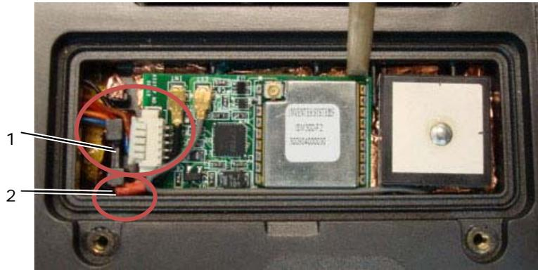
1 USB cable channel guide    2 GPS passthru antenna cable guide
