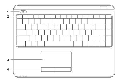
1 Power button and light — Turns the computer on or off when pressed. The light on the button indicates the power states.
