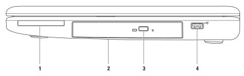
1 ExpressCard slot – Supports 34/54 mm wide ExpressCard. The computer ships with a plastic blank installed in the slot.
