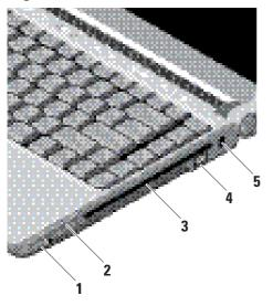
Wireless On/Off switch — Use this switch to rapidly turn all wireless devices Off or On such as WLAN cards and internal cards with Bluetooth wireless technology. The wireless switch may be in the Off position when your computer is shipped to you. To turn the switch On, slide the switch away from the front of the computer until it clicks into place.
