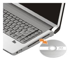
To eject a disc from the drive, gently touch the eject control. The control will flash to confirm a few seconds before ejecting the disc.
