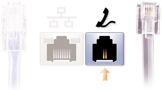
If your computer has an internal modem, connect the telephone cable to the modem connector and connect the other end of the cable to a telephone wall jack.
