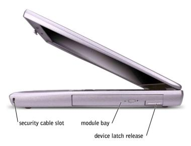
**SECURITY CABLE SLOT** — Lets you attach a commercially available antitheft device to the computer. For more information, see the instructions included with the device.
