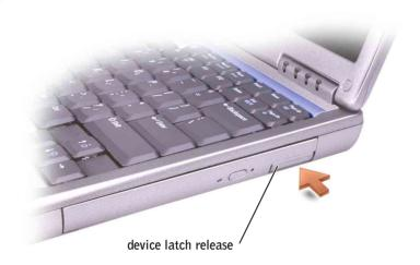
**5** Pull the device by the latch release to remove the device from the module bay.
