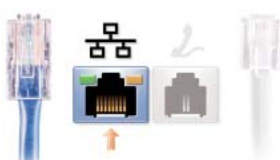
If your computer has a networking option, connect a separately purchased network cable to the network connector.
