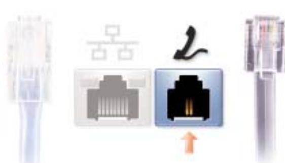
If your computer has an internal modem, connect the telephone cable to the modem connector and connect the other end of the cable to a telephone wall jack.
