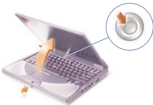
Open the display, and press the power button to turn on the computer. Follow the prompts on the screen to complete the operating system setup.
