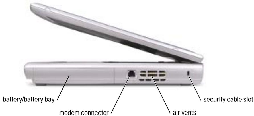
**BATTERY/BATTERY BAY** — When a battery is installed, you can use the computer without connecting the computer to an electrical outlet. See page 37.
