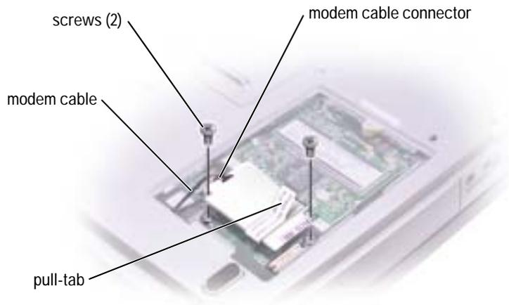
**2 Connect the modem cable to the modem.**
