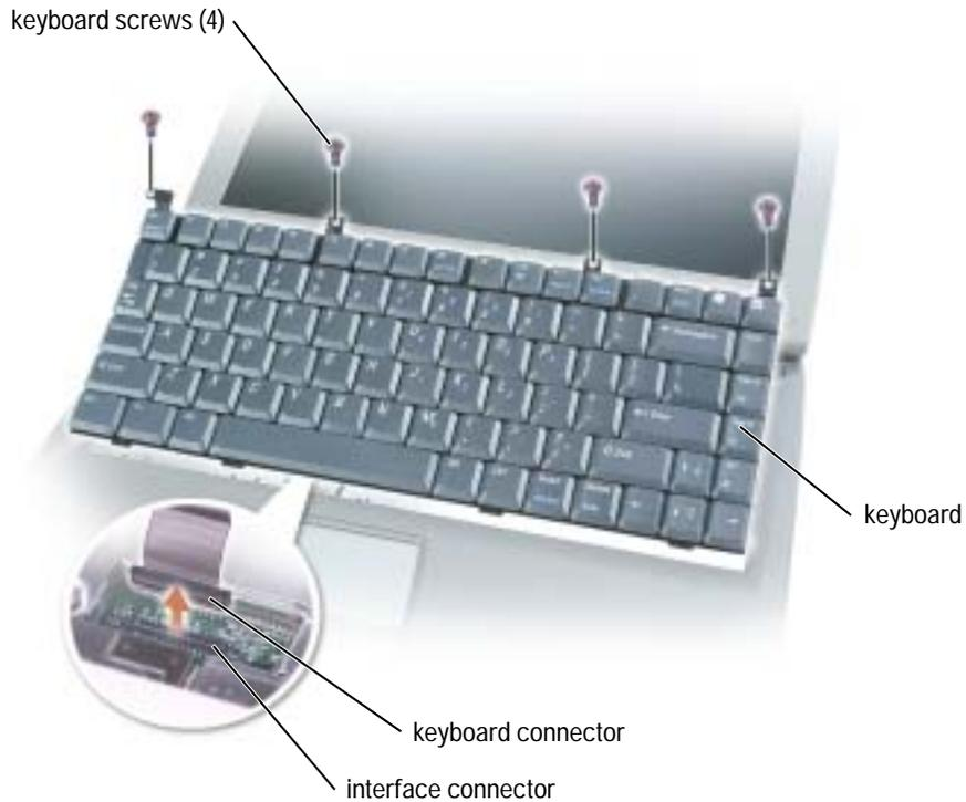
**7 Remove the keyboard from the bottom case.**
