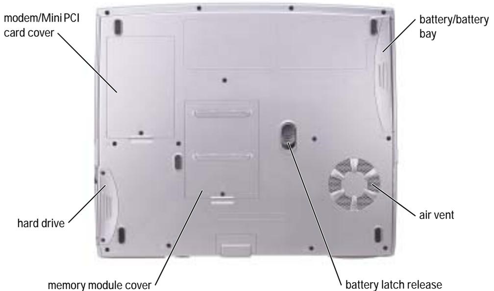
**MODEM/MINI PCI CARD COVER** — Covers the compartment that contains the modem and Mini PCI card. See page 82.
