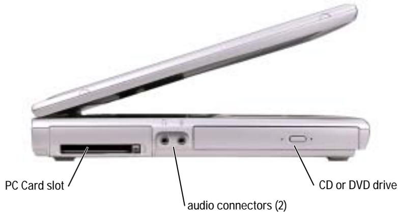
**PC CARD SLOT** — Supports one PC Card, such as a modem or network adapter. For more information, see "Using PC Cards" in the *Dell Inspiron Help* file. To access the help file, see page 16.
