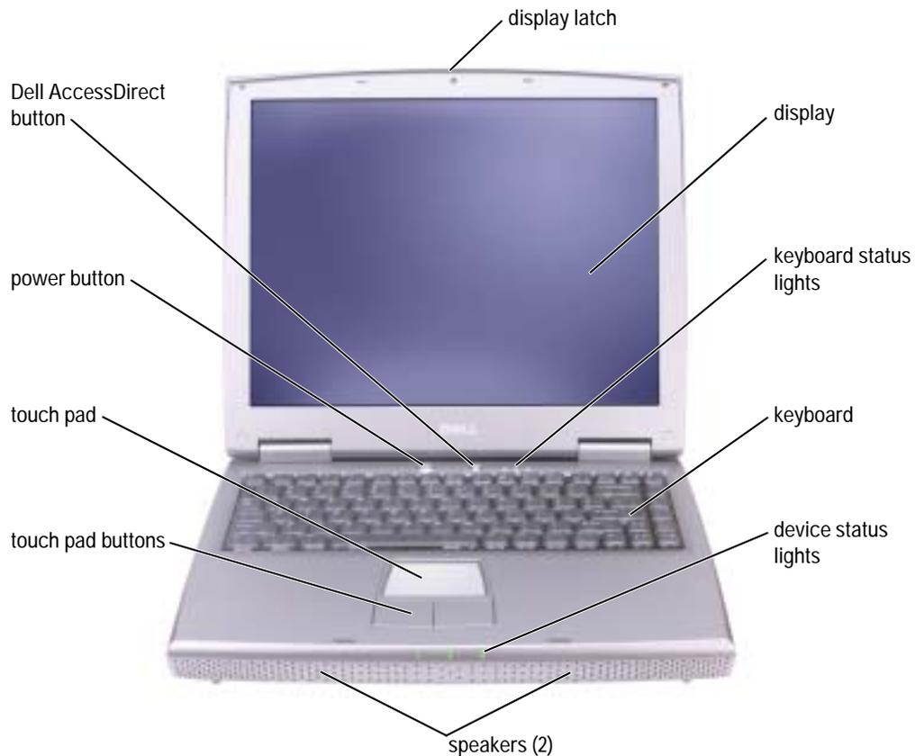
**DISPLAY LATCH** — Keeps the display closed.
