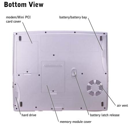
**MODEM/MINI PCI CARD COVER** — Covers the compartment that contains the modem and Mini PCI card. See page 102.
