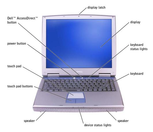
**DISPLAY LATCH** — Keeps the display closed.
