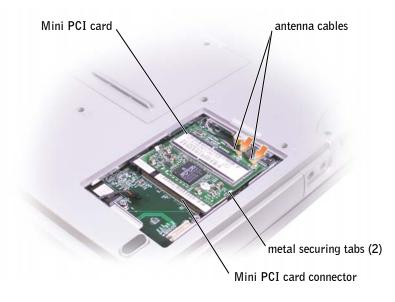
**NOTICE:** To avoid damaging the Mini PCI card, never place cables on top of or under the card.
