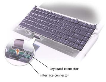
7 Remove the keyboard from the bottom case.
