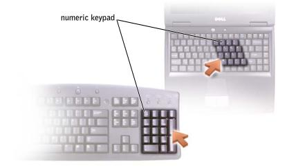
The numeric keypad functions like the numeric keypad on an external keyboard. Each key on the keypad has multiple functions. The keypad numbers and symbols are marked in blue on the right of the keypad keys.
