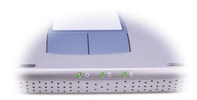
Turns on when you turn on the computer. Blinks or turns off in power management mode.
