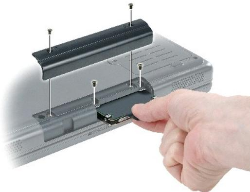
4. A black plastic strap is attached to the hard drive to assist in removal. Grasp the strap and pull straight out to remove the hard drive from computer.
