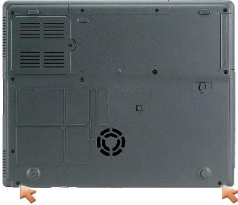
9. From the back of the computer, remove the two M2.5 x 8-mm screws labeled "D."
