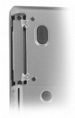
12. Remove the seven M2.5 x 8-mm screws from the bottom of the computer.
