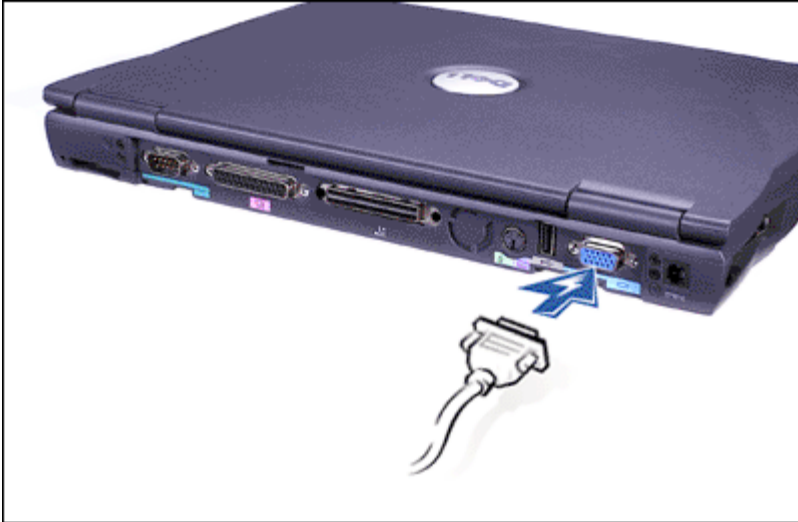
Figure 3. Connecting an External Monitor
