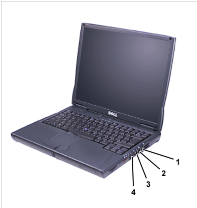
Figure 2. I/O Connectors on Right Side of Computer
