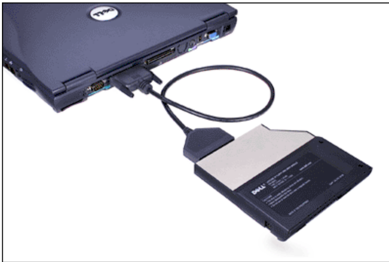
Figure 4. Using the Diskette Drive As an External Device
