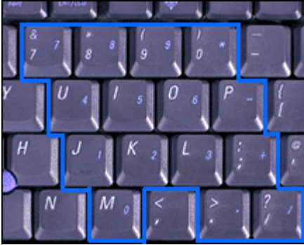
Figure 4. Embedded Numeric Keypad
