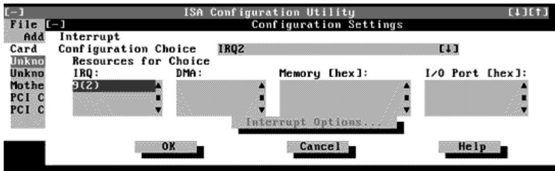
Figure 4-4. Configuration Settings Dialog Box for Assigning an IRQ Line
