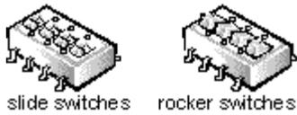
Each of these switches has two positions, or *settings* (usually *on* and *off*). To change the setting of a slide switch, use a small, pointed object such as a small screwdriver or a straightened paper clip to slide the switch to the proper position. To change the setting of a rocker switch, use the screwdriver or paper clip to press down on the appropriate side of the switch. In either case, do not use a pen, pencil, or other object that might leave a residue on the switch.
