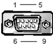
Figure B-3. Pin Numbers for the Serial Port Connectors
