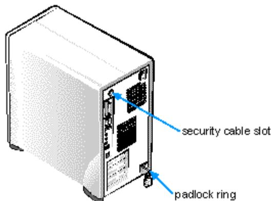
Figure 1-2. Security Cable Slot and Padlock Ring
