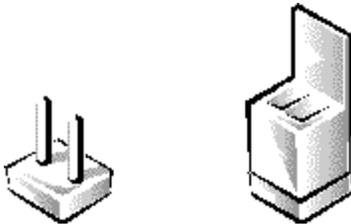
To change a jumper setting, pull the plug off its pin(s) and carefully fit it down onto the pin(s) indicated.
