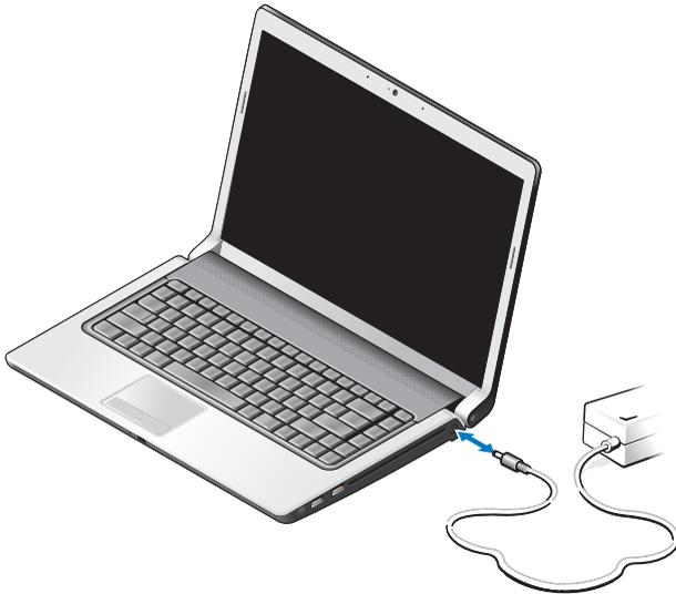
**⚠ CAUTION:** The AC adapter works with electrical outlets worldwide. However, power connectors and power strips vary among countries. Using an incompatible cable or improperly connecting the cable to the power strip or electrical outlet may cause fire or equipment damage.
