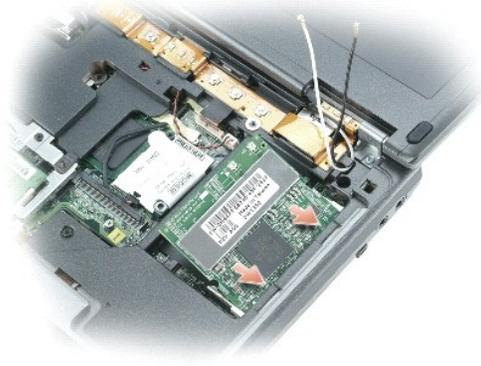
2. Connect the antenna cables to the Mini PCI card.
