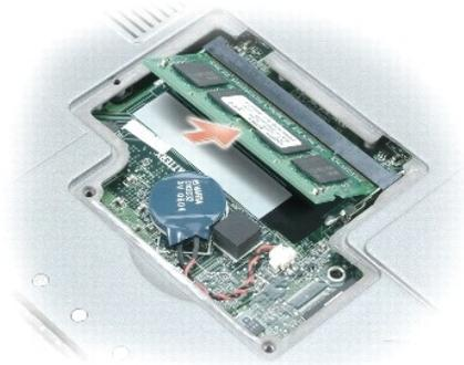
**NOTE:** If the memory module is not installed properly, the computer does not boot. No error message indicates this failure.
