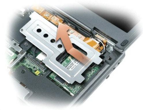
7. Disconnect the antenna cables from the Mini PCI card and re-route the cables so that they are clear of the computer base.
