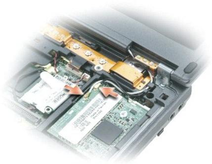
**🔧 NOTICE:** To prevent damage to the Mini PCI card connector, do not use tools to spread the securing clips that secure the card.
