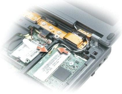
8. Pull up on the pull-tab to disconnect the display cable from the system board.
