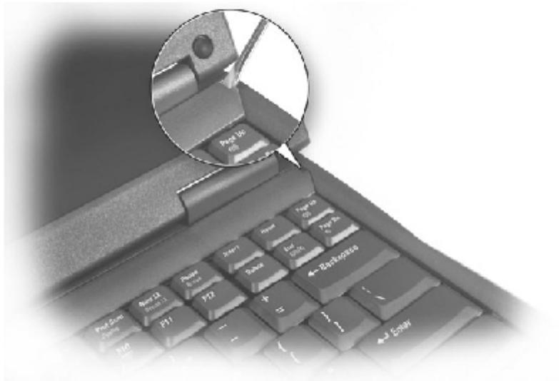
5. To release the keyboard from the palm rest, use a small, flat-blade screwdriver or plastic scribe to pull up on the scalloped edge of the blank key on the keyboard.
