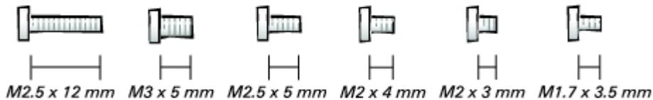
**NOTICE:** When reinstalling a screw, you must use a screw of the correct diameter and length. Make sure that the screw is properly aligned with its corresponding hole, and avoid over tightening.
