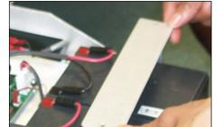
2 Detach the four battery terminal cable connectors and move them to the side.
