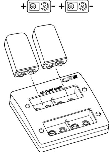
**WARNING: NEVER USE ALKALINE OR RECHARGEABLE ALKALINE BATTERIES.**
